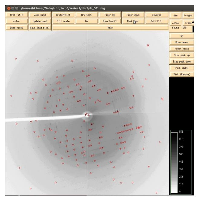
Because the default parameters for peak selection are usually sufficient, the alternate way perform a peak search is to switch to the *Index* tab and select *Peak search*. This will automatically select peaks from the first frame. It will also display the image if you have not previously done so.
