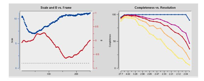
A good approach to determine the spacegroup is to initially scale the data in the lowest symmetry spacegroup for the crystal class and then select use the *Check Space Group* button. This assumes that CCP4 is installed and HKL-2000 is configured to use it, and uses the CCP4 program POINTLESS.
