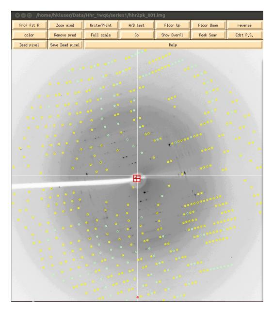
At this point, revisit the *Bravais Lattice* table and notice that the primitive orthorhombic class is the highest symmetry lattice type with a low correlation coefficient. Select this lattice and *Apply & Close* this window.
